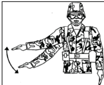
Figure E-26. Slow down engine(s) on indicated side
