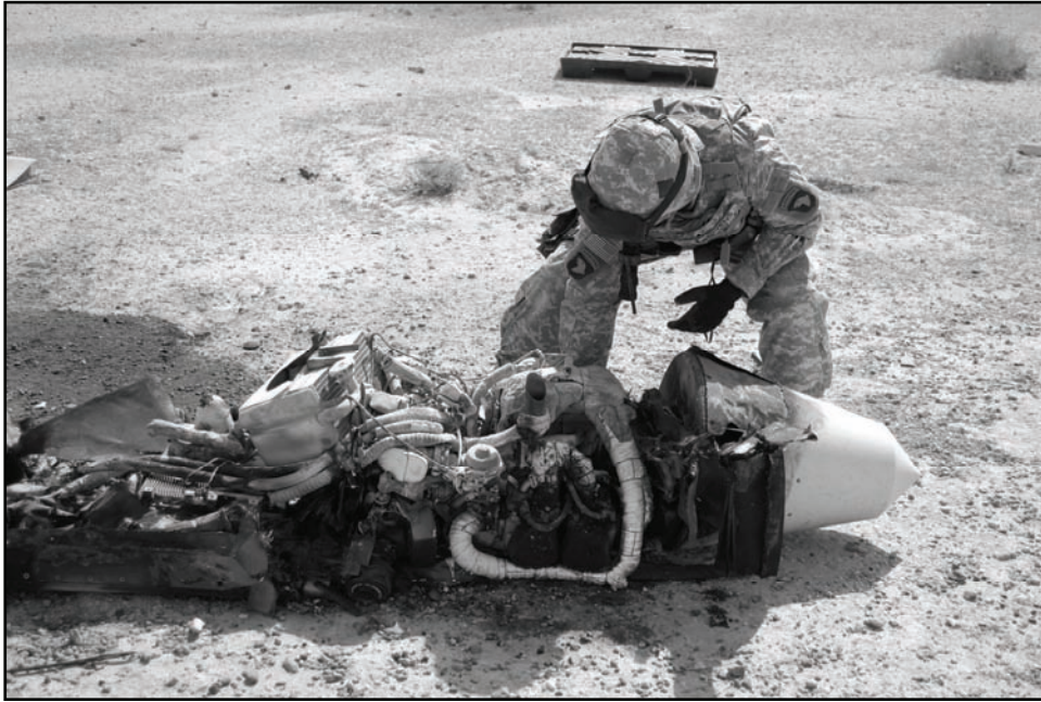
Figure 1-2. Downed aircraft recovery team examines unmanned aircraft engine
