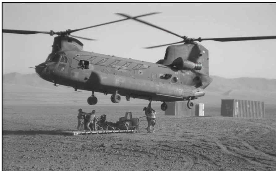
Figure 3-3. CH-47 performs salvage recovery utilizing a flat rack and military demountable containers
