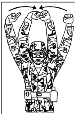
Figure E-28. Connect auxiliary power unit
