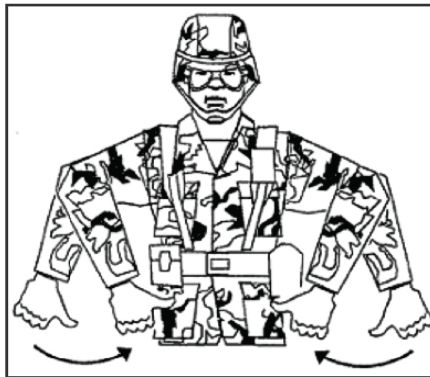
Figure E-30. Insert chocks/chocks inserted
