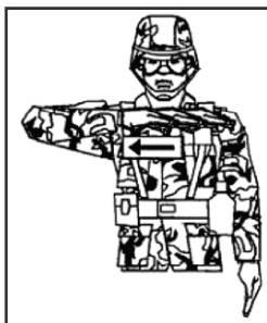
Figure E-27. Cut engine(s) or stop rotor(s)
