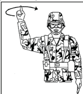
Figure E-15. Engage rotor(s)
