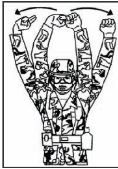
Figure E-29. Disconnect auxiliary power unit
